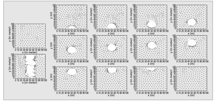
Figure 6. The two figures on the left illustrate that a mobile jammer can partition the network. The remaining figures depict the ability of a robust spatial retreats algorithm to repair the effect of a jammer passing through the coverage region.
