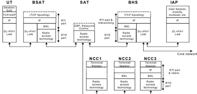
Fig. 2. BMSS protocol stack
