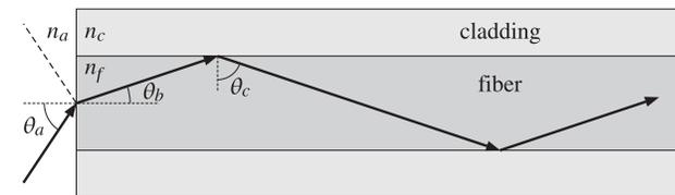
Fig. 7.5.5 Launching a beam into an optical fiber.
