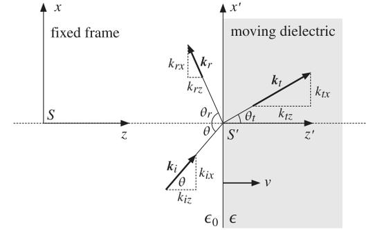
Fig. 7.12.1 Oblique reflection from a moving boundary.
