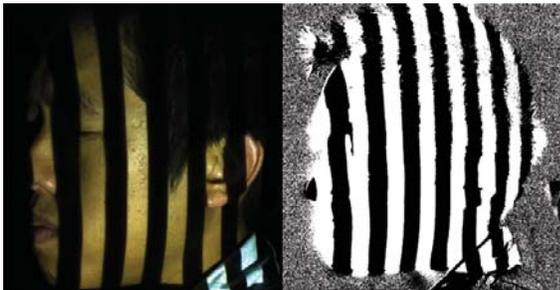
Figure 1. Original image with projected stripes (left). Ratio image (right). Clearly thresholding or edge detection in the original image will be problematic in the hair region. However, the ratio image shows strong unattenuated edges in this region.
