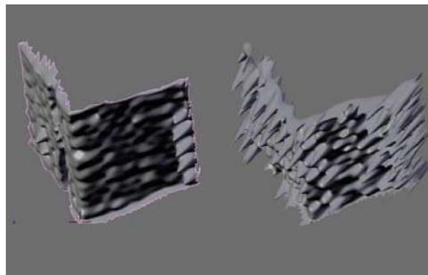
Figure 3. 3D Reconstruction using the ratio method (left) and using the Gray code (right). Notice that the darker regions have significant errors using the standard Gray code method.
