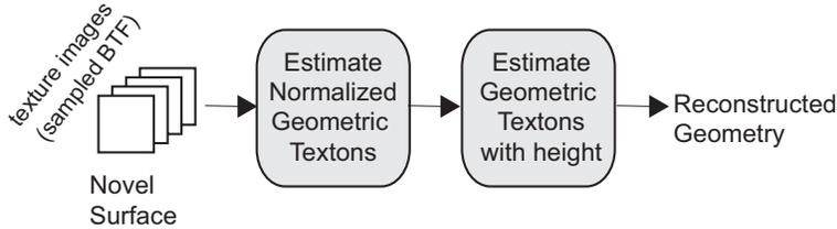
Fig. 9. Estimation of the local geometric texton. The sampled BTF of a novel surface is given. Then, the normalized geometric texton is estimated. Finally, the family of geometric textons with the same surface normal configuration but different heights is then considered and the closest match is used as the estimated geometric texton. To reconstruct geometry overlapping geometric textons are averaged.
