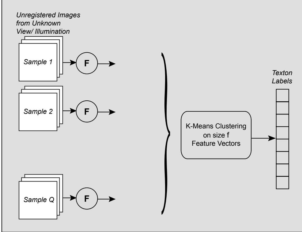
Fig. 5. Creation of the image texton library. The set of  $q$  unregistered texture images from the BTF of each of the  $Q$  samples are filtered with the filter bank  $F$  consisting of  $3 \times f$  filters, i.e.  $f$  filters for each of the three scales. The filter responses for each pixel are concatenated over scale to form feature vectors of size  $f$ . The feature space is clustered via k-means to determine the collection of key features, i.e the image texton library.
