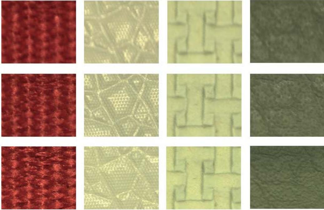
Fig. 17. Texture images for sample surfaces: (from left to right) canvas, rough plastic, rubber mat, and leather. Each image corresponds to a frontal view (i.e.  $\theta_v = 0$ ). The width is 10.5 mm and the height is 8.25mm. The top row corresponds to  $\theta_i = 12.1^\circ$ . For the middle row  $\theta_i = 0$ . For the last row  $\theta_i = -15.3^\circ$ . For each image  $\phi_i = 0$ , i.e. the illuminating ray intersects the mirror in the  $y - z$  plane.
