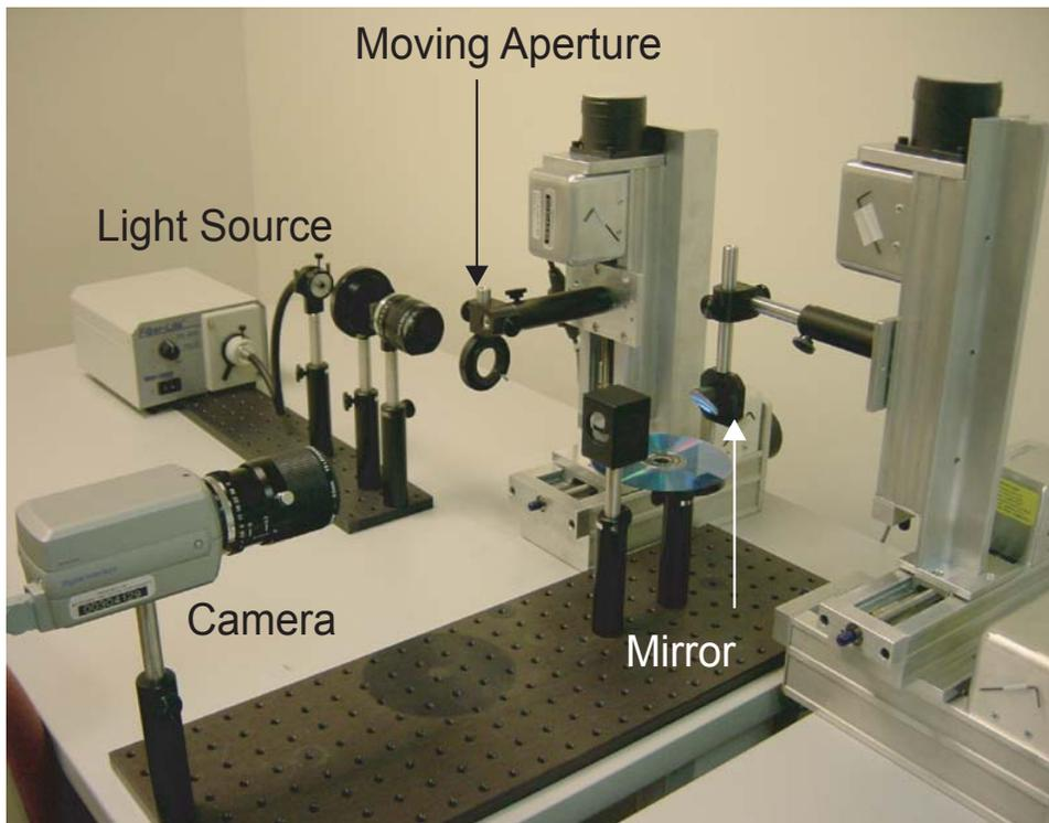
Fig. 15. Device prototype including camera, illumination source, collimating lens assembly, illumination aperture, beam splitter and off-axis concave parabolic mirror. A CD is the imaged sample placed at the focus of the mirror.
