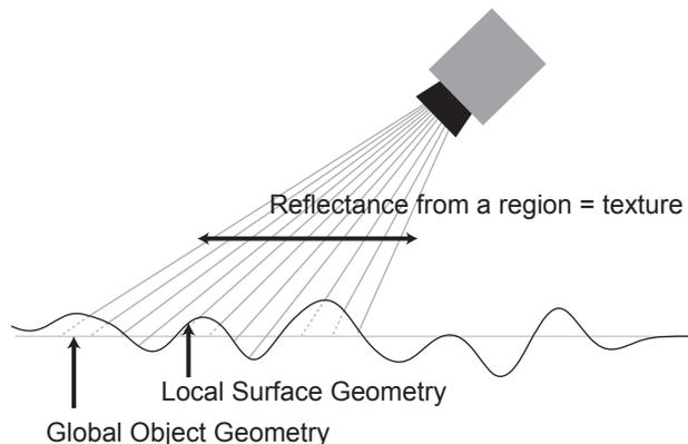
Fig. 3. Surface appearance or texture is the reflected light in a spatial region. We are interested in the case when the local geometry is not smooth and has some roughness. In general this fine-scale geometry is difficult to measure of model so image-based modeling techniques are useful.
