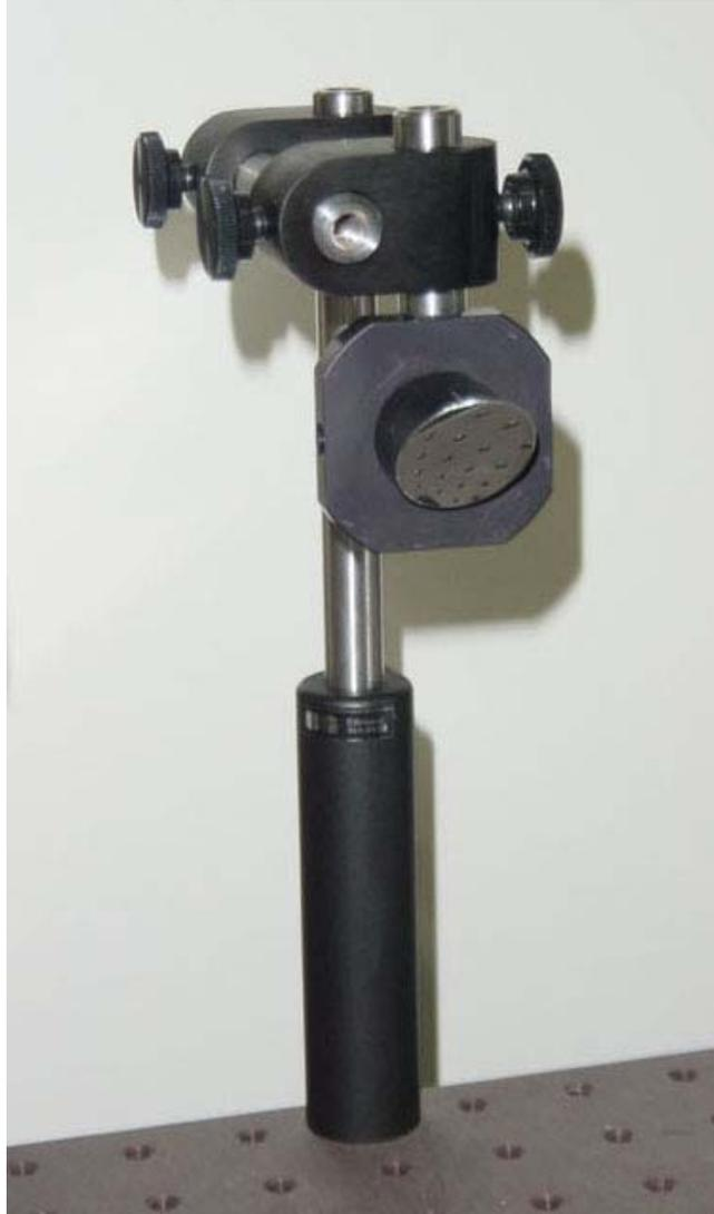
Fig. 16. Off-axis concave parabolic mirror used in prototype.
