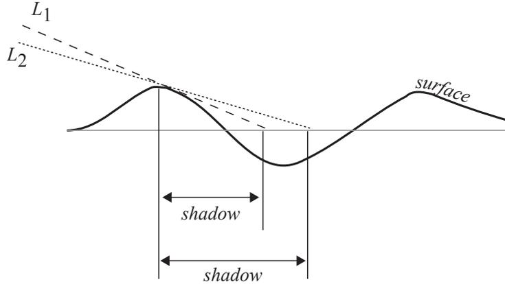
Fig. 8. An illustration of the creation of a shadow on a rough surface. The shadow length is determined by the illumination direction. As the illumination direction changes from  $L_1$  to  $L_2$  the shadow grows accordingly. The location, length, and continuous change of the shadow can be determined using geometric considerations. However, predicting cast shadows (that are not observed in the BTF sample images) is not possible with a purely image-based approach.
