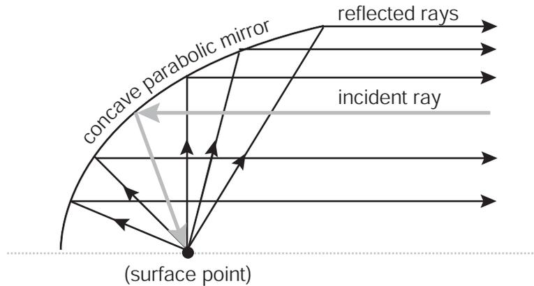
Fig. 13. The focusing property of a concave parabolic mirror is exploited to simultaneously measure reflected rays from a large range of angles over the hemisphere. The same mirror is used to direct the incident illumination ray to the sample at the desired angle.
