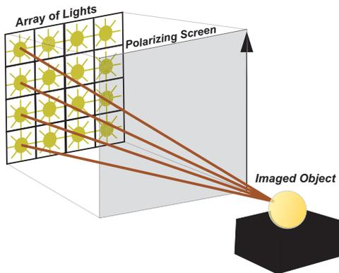
Figure 4. An object is imaged with multiple illumination directions and a polarized sheet is placed between the collection of light sources and the imaged object.
