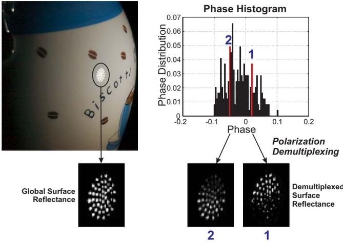
Figure 9. Multiplexing with one extended source. The jar is illuminated by one light source, and the phase distribution shows a single mode, as expected. By choosing two values for the phase, as shown by the two red bins, and performing polarization demultiplexing, the surface reflectance corresponding to two subdivisions of the light source is obtained. Notice that the demultiplexed specularities are indeed complementary.
