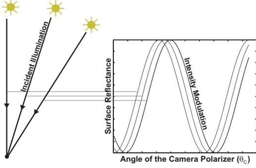
Figure 2. Because the light is polarized, there is a sinusoidal modulation on the intensity as a function of the camera polarizer angle. In addition, different angles of the incident illumination have modulation functions with different phases.
