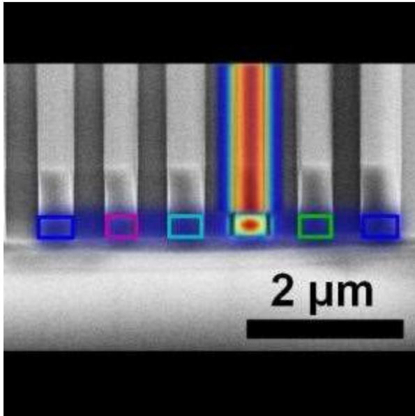
Image of a waveguide superlattice under a high-resolution electron microscope, artificially colored to show the optical field confined in one waveguide.
