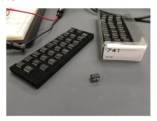
Sensitive parts should be moved around the lab and to or from your bench while still in the anti-static foam. Remove the parts from the foam only at your bench and on the mat.
