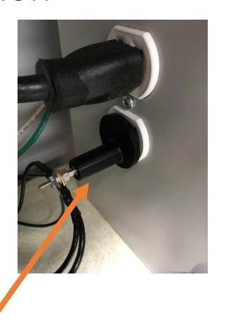
Grounding connections. Make sure they aren't disconnected
