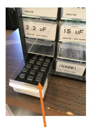
Sensitive parts should be stored in anti-static foam, and not lose in the parts bin.
