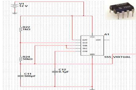
The output is taken from the timer's threshold and trigger pin instead of the output pin so that the result is a triangle wave rather than a square wave.
