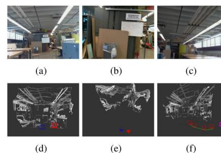
(d), and (e) show two different views of the 3D reconstruction of scene shown in (a), (b), and (c). The depth map for LSD-SLAM was initialized with a depth map from the Neural Network. (f) shows the reconstruction initialized with a random depth map.
