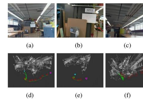
(d), (e), and (f) show three different views of the 3D reconstruction of scene shown in (a), (b), and (c). The blue camera frame represents one drone and the pink camera frame represent another. The green frames represent the pose graph for the blue drone, and the red frames represent the pose graph for the pink drone.
