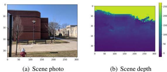
(b) shows the output of the depth prediction network for (a). The units of (b) are in meters and represent the distance from the camera each pixel is. Pixels that are lighter are further away. Distances greater than 70m are removed
