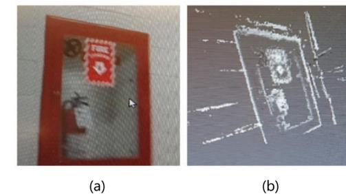
(b) shows the 3D reconstruction of (a) utilizing LSD-SLAM.
