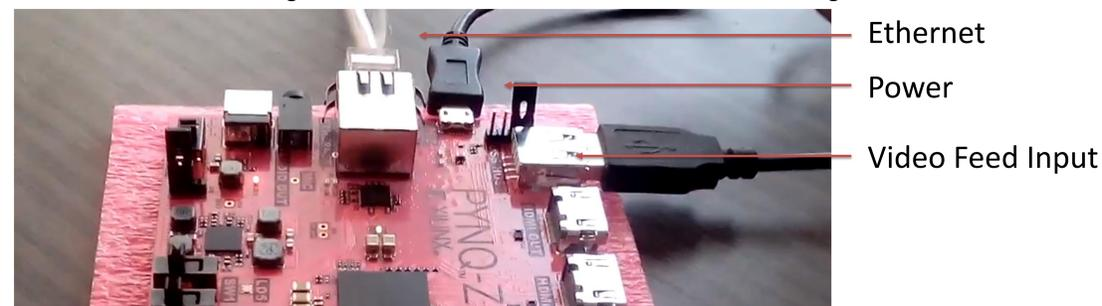
Figure 3: The realization of fig.2 on board
