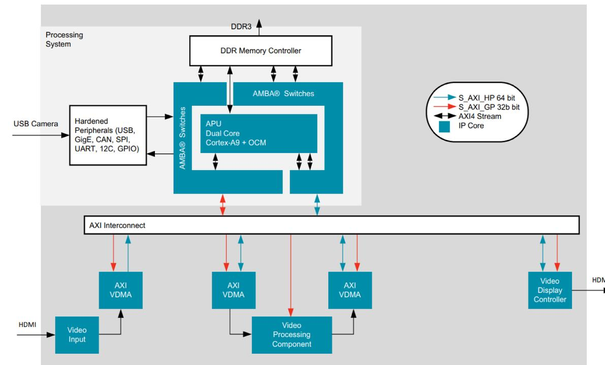
Figure 2: Frame-buffer Architecture for Video Processing<sup>[2]</sup>
