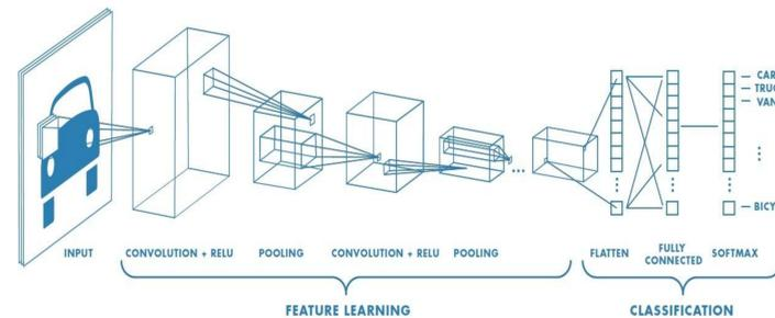
Figure 4. Convolutional Neural Network. The input goes through multiple streams of convolution and pooling during feature learning. The result then goes through the classification process, after which the image is identified as belonging to one of the pools in which the network was trained.
