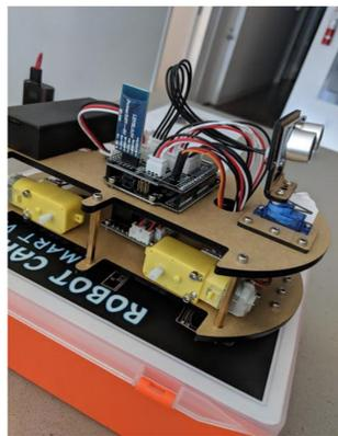
Fig 2. Autonomous Car. Arduino, Shield, and Sensors.
