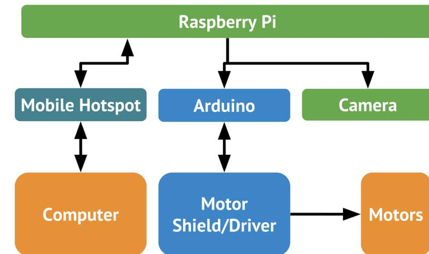
Figure 6. Hardware Interaction Diagram
