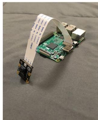
Fig 3. Raspberry Pi with Camera
