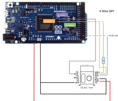
Figure 1: Transceiver circuit consisting of Arduino DUE and the A7105 Chip
