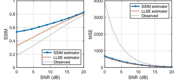
**Fig. 3:** (Natural image denoising with block size  $8 \times 8$ ) Comparisons of the SSIM-maximized linear estimator and LLSE estimator under the SSIM index and MSE metrics.
