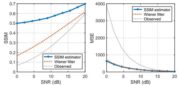
**Fig. 4:** (Natural image denoising with block size  $3 \times 3$ ) Comparisons of the SSIM-maximized linear estimator and LLSE estimator under the SSIM index and MSE metrics.
