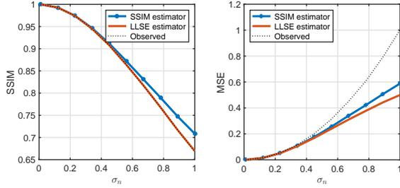
**Fig. 2:** (Gaussian source denoising) Comparisons of the SSIM-maximized linear estimator and LLSE estimator under the SSIM index and MSE metrics.
