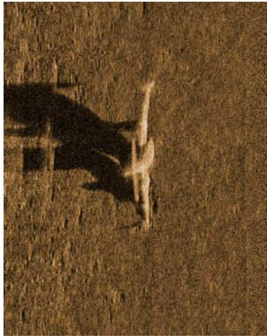
**Figure 1: Image of an aeroplane wreck obtained using side scan sonar released by National Oceanic and Atmospheric Administration (NOAA).**
