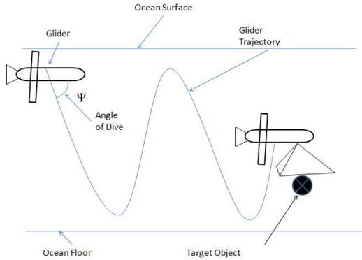
Figure 6: Sawtooth trajectory of the glider.
