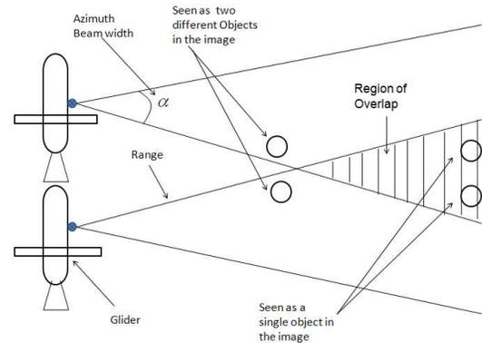
**Figure 2: Azimuth resolution or transverse resolution is the power to resolve the objects that lie in a line parallel to the path of the glider or the AUV.**
