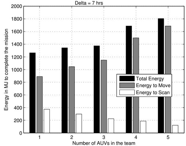
**Figure 12: Total energy of team of AUVs in MJ against the number of AUVs in the team when time bound  $\delta$  is 7 hr.**
