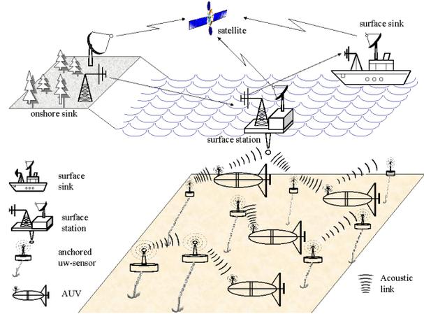
Figure 1: 3D Underwater Sensor Networks with AUVs.
