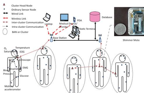
Fig. 1. Proposed Physical Network Architecture.
