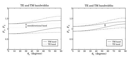
**Fig. 8.8.6** TM/TE bandgaps versus angle for  $n_H = 3$ ,  $n_L = 1.38$  and  $n_H = 2$ ,  $n_L = 1.38$ .
