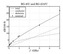
**Fig. 11.4.2** Attenuation coefficient  $\alpha$  versus frequency.
