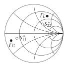
**Fig. 14.8.3** Optimum load and source reflection coefficients.
