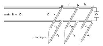
**Fig. 13.10.2** Triple stub tuner.
