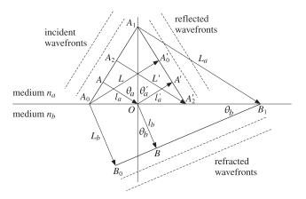
Fig. 7.14.1 Snel's laws of reflection and refraction.
