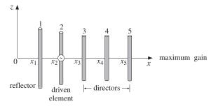
**Fig. 25.6.1** Five-element Yagi-Uda array.
