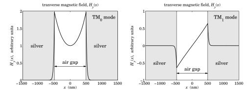
Fig. 10.7.2 Transverse magnetic field profiles for TM<sub>0</sub> and TM<sub>1</sub> plasmonic modes.
