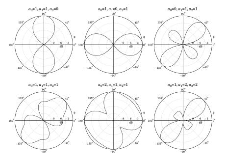
Fig. 22.3.4 Azimuthal gain patterns of two-dimensional array.
