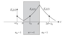
Fig. 8.6.2 Evanesenct wave amplification inside a negative-index medium.
