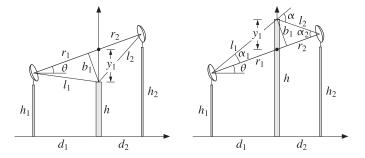
Fig. 18.14.3 Communicating antennas over an obstacle.
