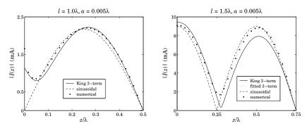
**Fig. 24.6.1** Three-term approximation for  $l = \lambda$  and  $l = 1.5\lambda$ .
