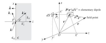
**Fig. 15.6.1** Elementary dipole at r' contributes to the local field at r.
