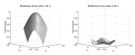
Fig. 21.6.4 Two-dimensional gain patterns from sides 1 & 3 and 2 & 4.
