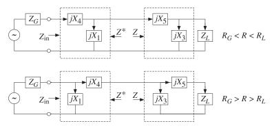
**Fig. 13.12.4** Double *L*-section networks.
