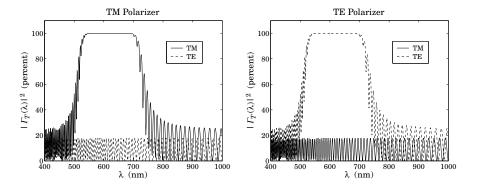
Fig. 8.13.4 TM and TE mirror polarizers.
