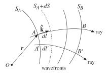
Fig. 7.13.1 Wavefront surfaces and rays.
