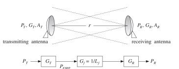
Fig. 16.6.1 Transmitting and receiving antennas.
