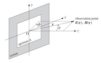
Fig. 18.4.1 Radiation fields from an aperture.
