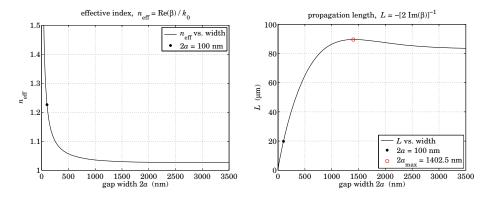
**Fig. 10.6.2** Effective index and propagation distance ( $\lambda_0 = 650 \text{ nm}$ ).
