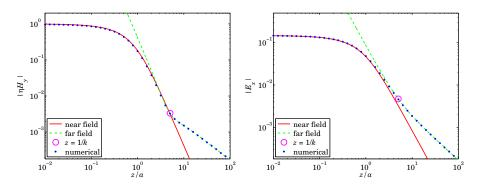
**Fig. 19.12.1** Fields  $\eta H_{\nu}$ ,  $E_x$  at x = y = 0 versus distance z from aperture.
