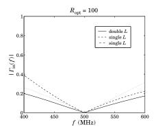
**Fig. 13.12.5** Comparison of single and double *L*-section networks.
