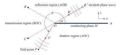
Fig. 19.10.1 Plane wave incident on conducting half-plane.
