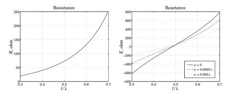
Fig. 17.3.1 Input impedance of standing-wave dipole antenna.
