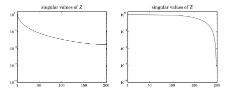
**Fig. 24.14.2** Singular values of the impedance matrices  $\mathcal{Z}$  and  $\bar{Z}$  for N=2M+1=201.
