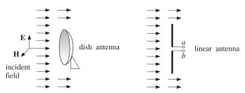
Fig. 16.3.1 Effective area of an antenna.
