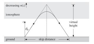
Fig. 7.15.2 Ionospheric refraction.
