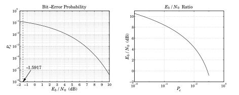
**Fig. 16.9.1**  $P_e$  versus  $E_h/N_0$ , and its inverse, for a BPSK system.
