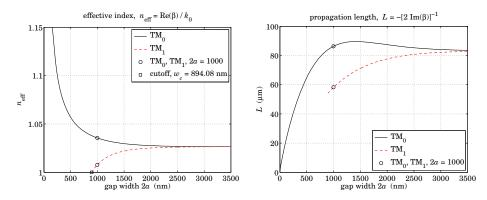
**Fig. 10.7.1** Effective index and propagation distance for TM<sub>0</sub> and TM<sub>1</sub> plasmonic modes.
