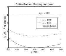
Fig. 5.5.3 Reflectance over the visible spectrum.
