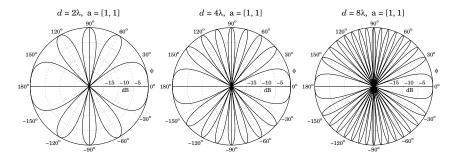
Fig. 22.3.2 Grating lobes of two-element isotropic array.
