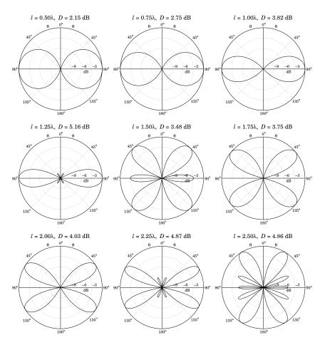
Fig. 17.4.2 Standing-wave dipole antenna patterns and directivities.
