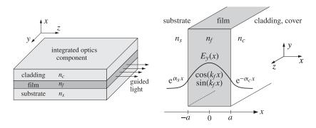
Fig. 9.12.1 Three-layer asymmetric dielectric slab waveguide.
