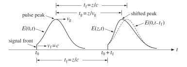
**Fig. 3.2.1** Causal pulse propagation, but with superluminal group velocity  $(v_a > c)$ .
