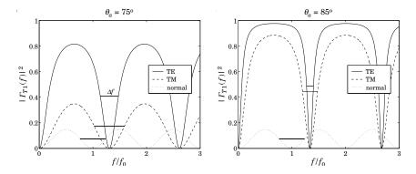
Fig. 8.3.2 TE and TM reflectances of half-wavelength slab.
