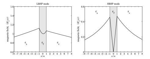
**Fig. 10.13.3** Magnetic field profiles, 2a = 20 nm film.
