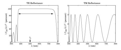
**Fig. 8.9.2** Polarizer with  $n_H = 2.3$  and  $n_L = 1.25$ .
