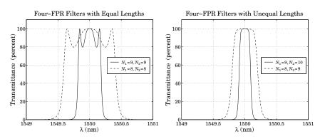
**Fig. 6.5.4** Transmission filters with four FPRs of equal and unequal lengths.
