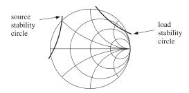
**Fig. 14.5.3** Load and source stability circles at 1 GHz.
