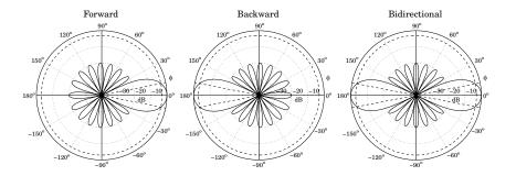
Fig. 23.9.6 Forward, backward, and bidirectional endfire designs.
