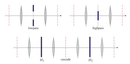
Fig. 20.11.3 Lowpass, highpass, and cascaded filter examples.
