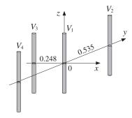
**Fig. 25.5.5** Four-element parasitic array.
