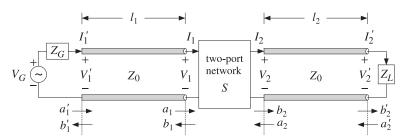
Fig. 14.1.3 Two-port network under test.
