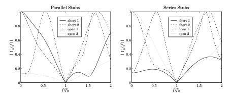
Fig. 13.8.3 Reflection response of single stub matching solutions.
