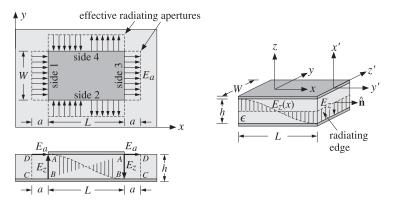
**Fig. 21.6.2** Aperture models for microstrip antenna.
