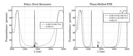
Fig. 6.5.1 Narrowband FPR transmission filters.
