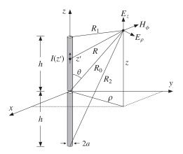
Fig. 25.1.1 Fields of a thin wire antenna.
