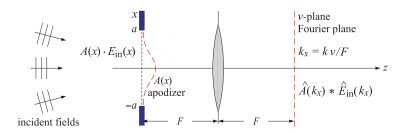
Fig. 20.12.1 Apodization or windowing.
