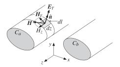
Fig. 9.2.1 Conductor surface absorbs power from the propagating fields.
