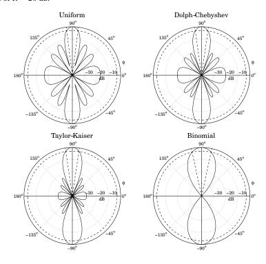
**Fig. 23.7.1** Narrow beam design examples.
