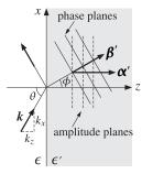
Fig. 7.9.1 Constant-phase and constant-amplitude planes for refracted wave.
