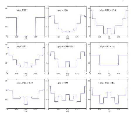
**Fig. 20.2.2** Magnitude  $|E(x, z_{pq})|$  versus x, over one period,  $0 \le x \le d$ .
