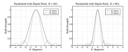
Fig. 21.10.1 Parabolic reflector patterns with dipole feed.
