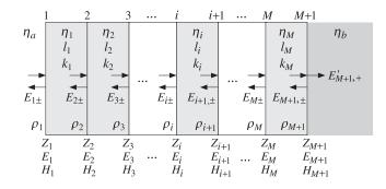
Fig. 6.1.1 Multilayer dielectric slab structure.
