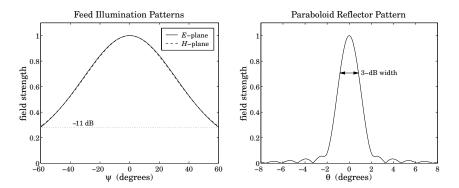
Fig. 21.10.3 Feed and reflector radiation patterns.
