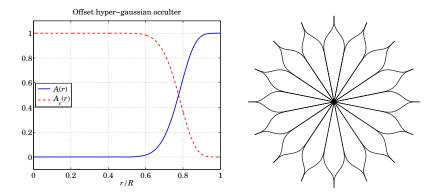
Fig. 20.20.3 Occulting apodizer and its star-shaped realization.
