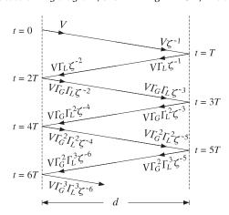
Fig. 11.15.2 Lattice timing diagram.
