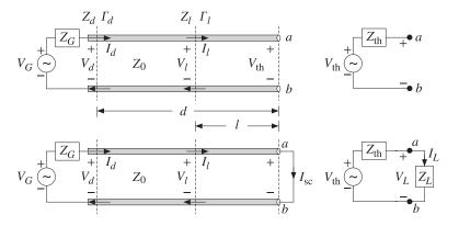
Fig. 11.11.1 Open- and short-circuited line and Thévenin-equivalent circuit.
