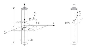
Fig. 24.1.1 Thin-wire model of cylindrical antenna.
