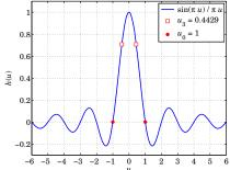
Fig. 20.11.4 2-D and 1-D lowpass inpulse responses.
