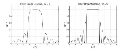
Fig. 12.5.2 Reflectance of fiber Bragg gratings.
