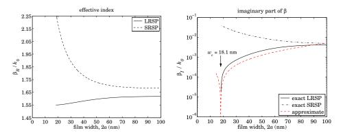
**Fig. 10.13.2** Real and imaginary parts of wavenumber  $\beta$ .
