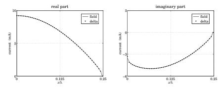
Fig. 24.13.1 Comparison of delta-gap and field solutions for a half-wave dipole.
