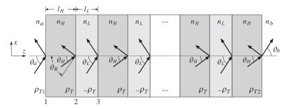
Fig. 8.8.1 Dielectric mirror at oblique incidence.
