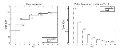
Fig. 11.15.3 Transient step and pulse responses of a terminated line.
