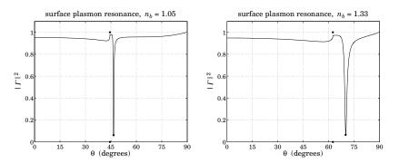
**Fig. 8.5.7** Shift of the resonance angle with the refractive index  $n_h$ .
