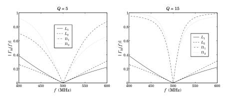
**Fig. 13.12.3** Comparison of *L*-section and  $\Pi$ -section matching.
