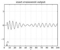
Fig. 3.4.2 Transient and steady-state response for evanescent sinusoids.
