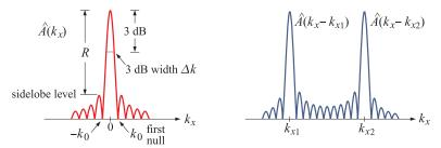
Fig. 20.12.2 Basic parameters of an apodizing function.
