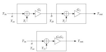
Fig. 16.8.2 Equivalent noise model of two cascaded devices.
