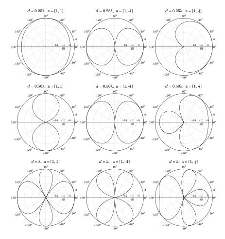
Fig. 22.3.1 Azimuthal gain patterns of two-element isotropic array.
