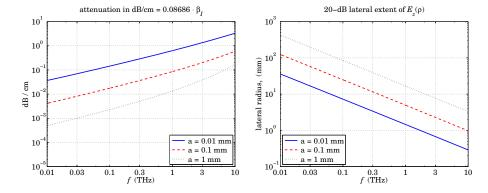
Fig. 10.15.4 Attenuations and 20-dB lateral distances vs. frequency.
