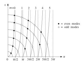
Fig. 9.11.2 Even and odd TE modes at different frequencies.
