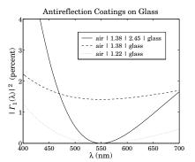
Fig. 6.2.1 Two-slab reflectionless coating.
