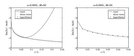
**Fig. 24.10.3** Logarithmic behavior of the solution near z = 0.
