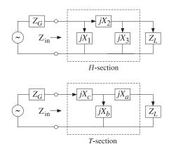
**Fig. 13.12.1**  $\Pi$ - and T-section matching networks.
