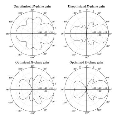
Fig. 25.6.5 Gains of six-element Yagi-Uda array.
