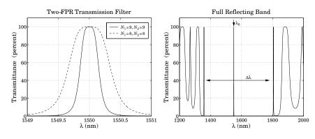
Fig. 6.5.2 Narrow-band transmission filter made with two FPRs.
