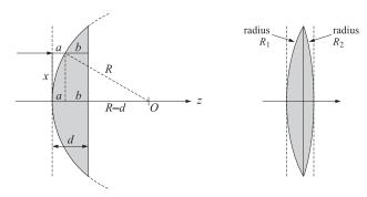
**Fig. 20.5.1** Transmittance of a thin spherical lens.
