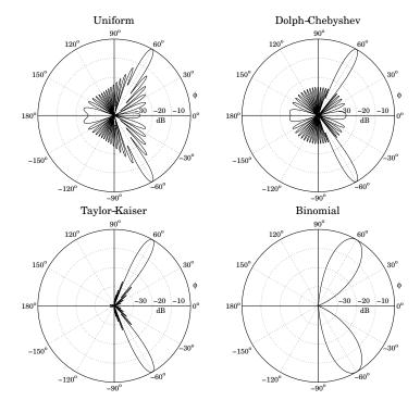
Fig. 23.7.2 Comparison of steered 21-element narrow-beam arrays.
