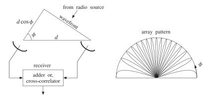
Fig. 22.6.1 Two-element interferometer and typical angular pattern.
