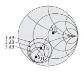
Fig. 14.10.1 Unilateral input gain circles.
