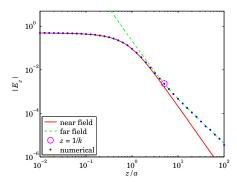
**Fig. 19.12.2** Field  $E_z$  at x = v = 0 versus distance z from aperture.
