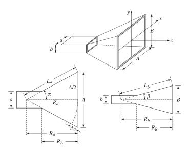
**Fig. 21.2.2** The geometry of the pyramidal horn requires  $R_A = R_B$ .
