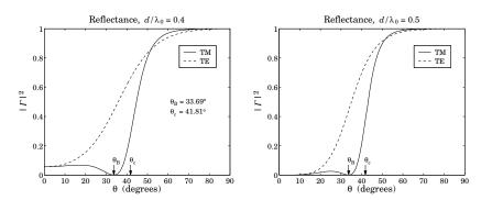
**Fig. 8.4.4** Reflectance versus angle of incidence.
