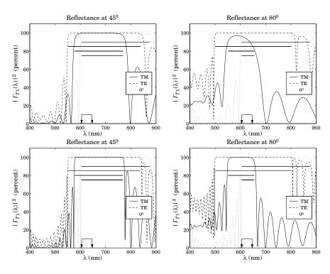
Fig. 8.8.10 Omnidirectional mirror over visible band.
