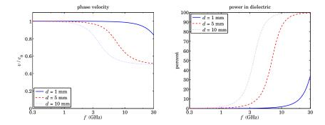
Fig. 10.20.2 Phase velocities and power in dielectric.
