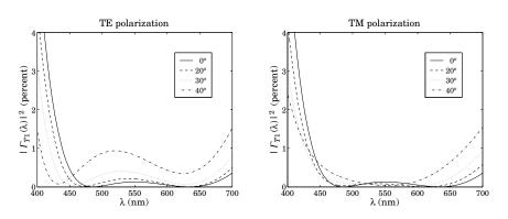
Fig. 8.7.3 Three-layer antireflection coating at oblique incidence.
