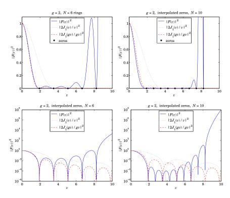
**Fig. 20.21.3** Superresolution gain q = 2, with 5 zeros of  $J_1(qv) = 0$ , and interpolated zeros.
