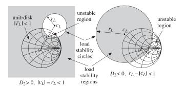
Fig. 14.5.2 Load stability regions in potentially unstable case.
