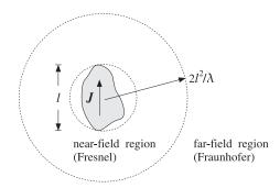
Fig. 15.7.2 Far-field and near-field radiation zones.
