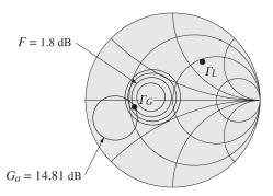
Fig. 14.12.3 Maximum available gain for given noise figure.
