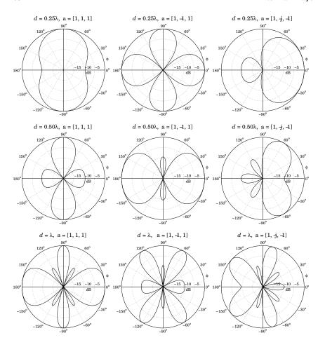
Fig. 22.3.3 Azimuthal gains of three-element isotropic array.
