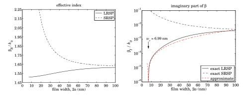
**Fig. 10.13.4** Real and imaginary parts of wavenumber  $\beta$ .
