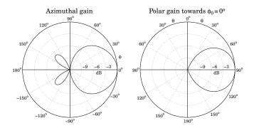
**Fig. 25.5.6** *H*-plane and *E*-plane radiation patterns,  $V = [1, 0, 0, 0]^T$ .
