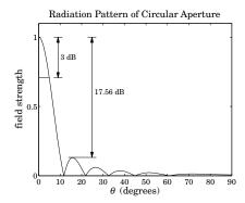
**Fig. 18.9.2** Radiation pattern of circular aperture ( $a = 3\lambda$ ).
