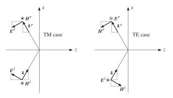
Fig. 19.9.2 Plane-wave components of incident and reflected waves.
