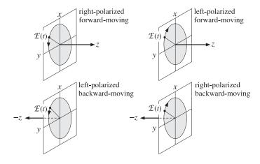
Fig. 2.5.1 Left and right circular polarizations.
