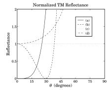
Fig. 8.11.2 TM reflectances normalized at normal incidence.
