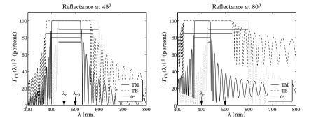
**Fig. 8.8.2** TM and TE reflectances for  $n_H = 2.32$ ,  $n_L = 1.38$ .
