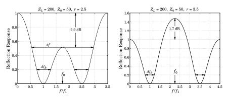
**Fig. 13.4.3** Dual-band transformers at frequencies  $\{f_1, 2.5f_1\}$  and  $\{f_1, 3.5f_1\}$ .
