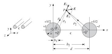
Fig. 11.5.1 Two-wire transmission line.
