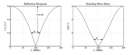
Fig. 13.3.2 Reflection response and line SWR of single-section transformer.
