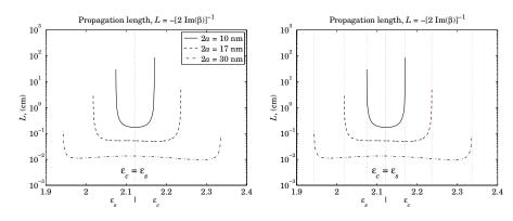
**Fig. 10.13.5** Propagation length *L* vs. permittivity  $\varepsilon_c$ .
