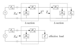
**Fig. 13.12.2** Equivalent *L*-section networks.
