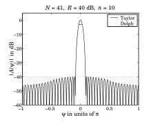
**Fig. 23.12.1** Taylor  $\bar{n}$  line source array design.
