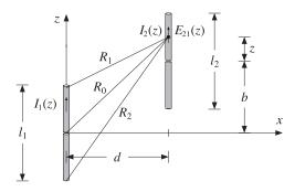
Fig. 25.3.1 Parallel linear dipoles.
