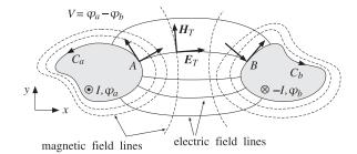
Fig. 11.1.1 Two-conductor transmission line.
