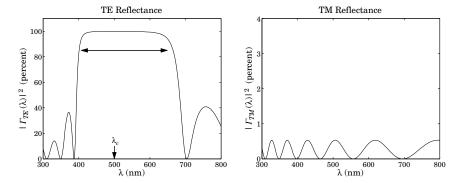
**Fig. 8.9.3** Polarizer with  $n_H = 2.04$  and  $n_L = 1.385$ .
