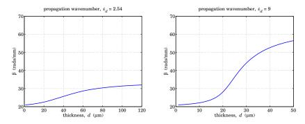
Fig. 10.19.11 Propagation wavenumbers vs. thickness at 1 THz.
