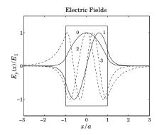
**Fig. 9.11.3** TE modes and corresponding *E*-field patterns.
