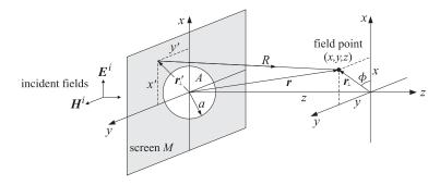
**Fig. 19.11.1** Circular aperture at z = 0, incident fields from z < 0, field point at  $z \ge 0$ .
