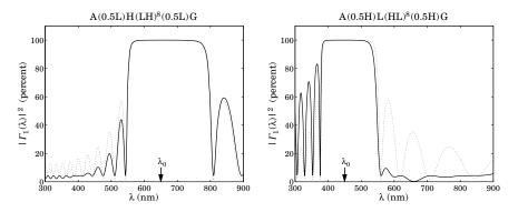
**Fig. 6.3.5** Short- and long-pass wavelength filters.
