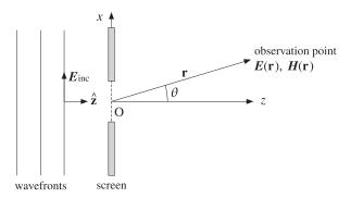
**Fig. 18.5.1** Uniform plane wave incident on an aperture.
