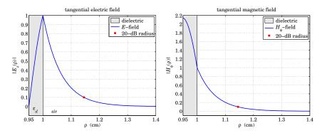
Fig. 10.19.2 Tangential electric and magnetic fields.
