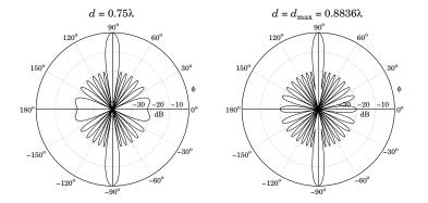
**Fig. 23.9.3** Chebyshev arrays with N = 9, R = 20 dB,  $d = 3\lambda/4$  and  $d = 0.8836\lambda$ .
