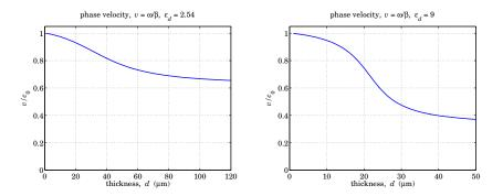
Fig. 10.19.12 Phase velocity vs. thickness at 1 THz.
