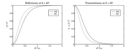
**Fig. 8.4.3** Reflectance and transmittance versus thickness *d*.
