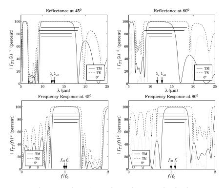
Fig. 8.8.8 Nine-layer Te/PS omnidirectional mirror over the infrared.
