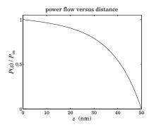
**Fig. 8.5.5** Power flow within metal layer at the resonance angle  $\theta_{res} = 43.58^{\circ}$ .
