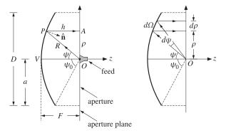
Fig. 21.7.1 Parabolic reflector antenna with feed at the focus.
