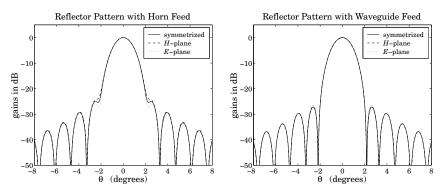
**Fig. 21.10.4** Exact and approximate reflector radiation patterns.
