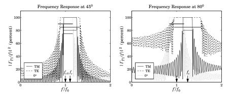
**Fig. 8.8.3** TM and TE frequency responses for  $n_H = 2.32$ ,  $n_I = 1.38$ .
