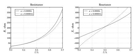
Fig. 24.10.6 Input impedance versus antenna length.
