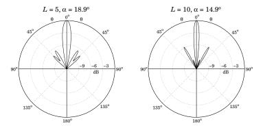
Fig. 17.7.3 Traveling-wave vee antenna gains in dB.
