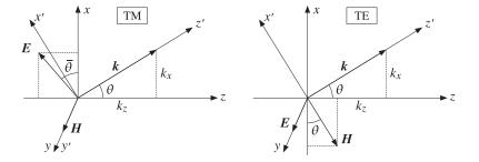
Fig. 4.6.1 Uniform plane waves in a birefringent medium.
