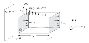
Fig. 2.6.1 Power flow in lossy dielectric.
