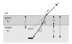
7.10 An underwater object is viewed from air at an angle  $\theta$  through two glass plates of refractive indices  $n_1, n_2$  and thicknesses  $z_1, z_2$ , as shown below. Let  $z_3$  be the depth of the object within the water.
