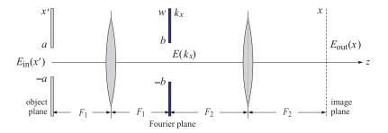
Fig. 20.22.3 Bandlimited optical system.
