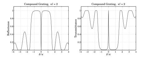
Fig. 12.5.4 Quarter-wave phase-shifted fiber Bragg grating.
