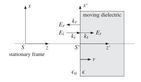
Fig. 5.8.1 Reflection and transmission at a moving boundary.
