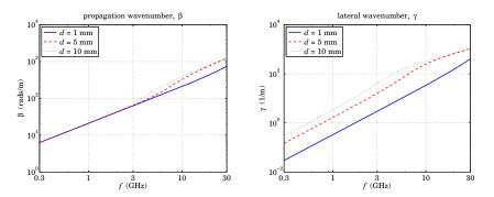
**Fig. 10.20.1** Propagation and lateral wavenumbers,  $\beta$ ,  $\gamma$ , vs. frequency.
