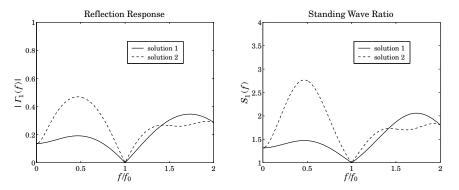
Fig. 13.7.2 Reflection response of two-section series transformer.
