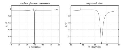
**Fig. 8.5.6** Surface plasmon resonance at the optimum thickness  $d = d_{opt}$ .
