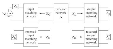
Fig. 13.13.3 Designing input and output matching networks for a two-port.
