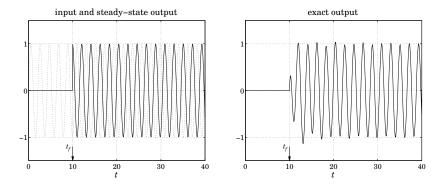
Fig. 3.4.1 Transient and steady-state sinusoidal response.
