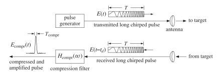
Fig. 3.10.1 Chirp radar system.
