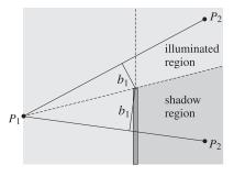
Fig. 18.14.1 Illuminated and shadow regions in straight-edge diffraction.
