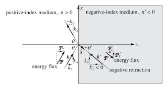
Fig. 7.16.1 Refraction into a negative-index medium.
