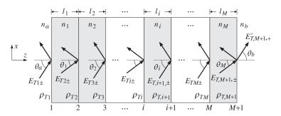
Fig. 8.1.1 Oblique incidence on multilayer dielectric structure.
