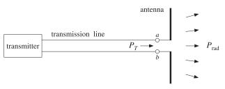
**Fig. 16.2.1** Power delivered to an antenna versus power radiated.
