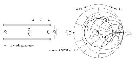
Fig. 11.14.3 Moving towards the generator along a constant SWR circle.
