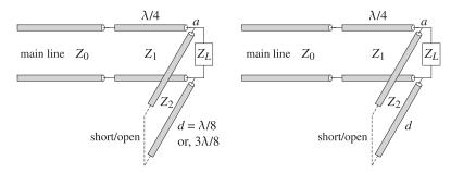
Fig. 13.6.1 Matching with a quarter-wavelength section and a shunt stub.
