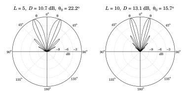
Fig. 17.6.2 Traveling-wave antenna gain examples.
