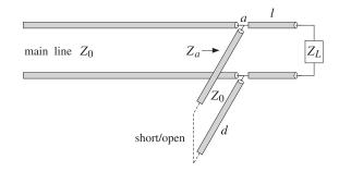
Fig. 13.8.1 Parallel connection of single stub tuner.
