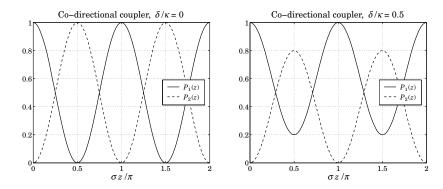
Fig. 12.4.2 Power exchange in co-directional couplers.
