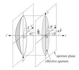
Fig. 21.7.2 Parabolic antenna and its projected effective aperture.
