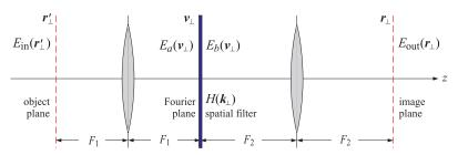
Fig. 20.11.1 4F optical processor.
