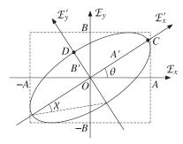
Fig. 2.5.2 General polarization ellipse.
