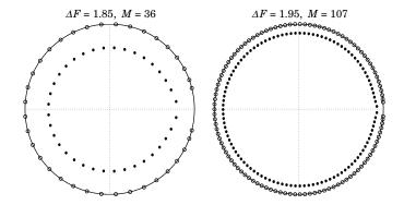
**Fig. 6.8.3** Zero patterns of B(z) (open circles) and A(z) (filled circles), for A=30 dB.
