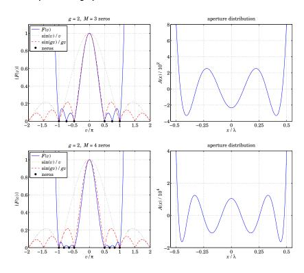
**Fig. 20.21.5** Superresolution gain q = 2, with M = 3, 4 zeros, visible region  $-\pi \le \nu \le \pi$ .
