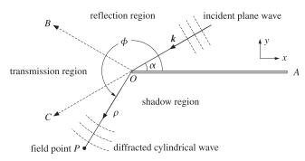
Fig. 18.15.1 Plane wave incident on conducting half-plane.
