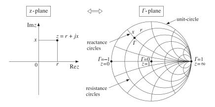
**Fig. 11.14.1** Mapping between *z*-plane and *Γ*-plane.
