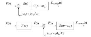
Fig. 3.10.2 Pulse compression filter.
