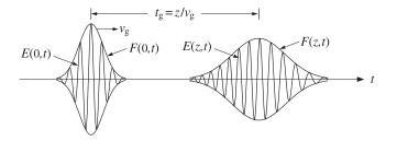
**Fig. 3.6.1** Pulse spreading and chirping.
