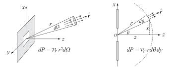
Fig. 19.7.1 Radiated power from 2-D and 1-D apertures.
