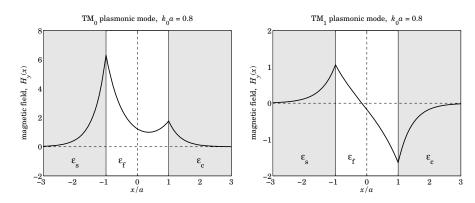
**Fig. 10.4.8** Magnetic field profiles of  $TM_0$  and  $TM_1$  modes for  $k_0a = 0.80$ . Region 3.
