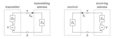
Fig. 16.4.1 Circuit equivalents of transmitting and receiving antennas.
