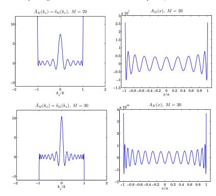
**Fig. 20.22.1** Optimum superdirective aperture, with M = 20, 30.
