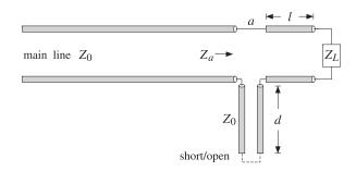
Fig. 13.8.2 Series connection of single stub tuner.
