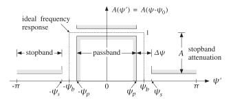
Fig. 23.4.1 Specifications of equivalent lowpass response.
