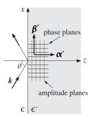
**Fig. 7.8.1** Constant-phase and constant-amplitude planes for total internal reflection ( $\theta \ge \theta_c$ ).
