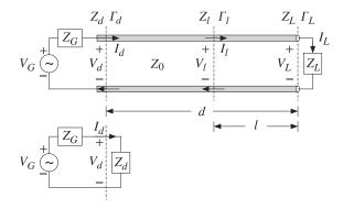
Fig. 11.9.1 Terminated line and equivalent circuit.
