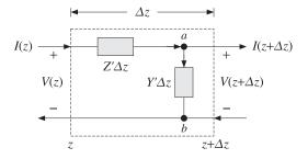
Fig. 11.6.1 Distributed parameter model of a transmission line.
