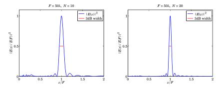
**Fig. 20.3.2** Focusing by Fresnel zone plate.
