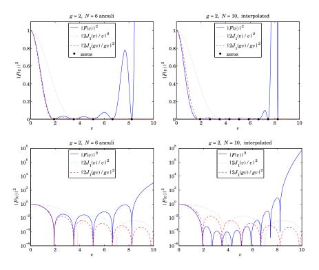
**Fig. 20.21.4** Superresolution gain g = 2, with 5 zeros of  $J_1(gv) = 0$ , and interpolated zeros.
