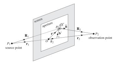
**Fig. 18.13.1** Fresnel diffraction through rectangular aperture.
