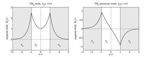
**Fig. 10.5.5** Magnetic field profiles of  $TM_0$  and  $TM_1$  modes for  $k_0a = 0.80$ . Symmetric guide.
