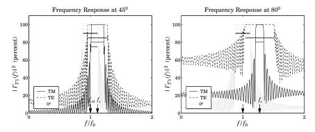
**Fig. 8.8.4** TM and TE reflectances for  $n_H = 2$ ,  $n_L = 1.38$ .
