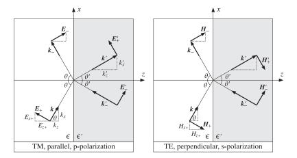
**Fig. 7.1.1** Oblique incidence for TM- and TE-polarized waves.
