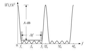
Fig. 6.8.1 Reflectance specifications for Chebyshev design.
