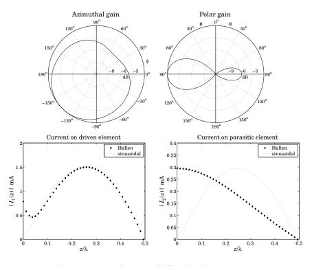
**Fig. 25.7.2** Gains and currents of full-wavelength parasitic array.
