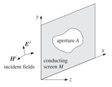
Fig. 19.9.1 Aperture in planar conducting screen.
