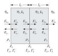
Fig. 5.7.1 Two dielectric slabs.
