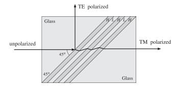
Fig. 8.9.1 Polarizing beam splitter.
