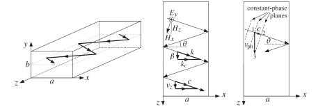
**Fig. 9.9.1** Reflection model of  $TE_{10}$  mode.
