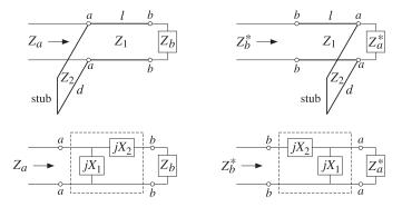
**Fig. 13.13.2** Examples of reversed matching networks.
