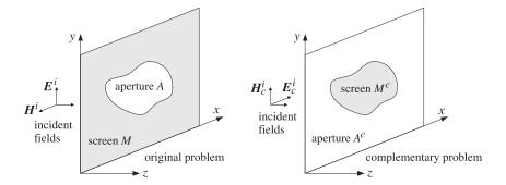
Fig. 19.13.1 Original and complementary metallic screen and aperture.
