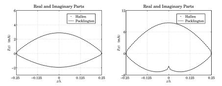
Fig. 24.14.1 Comparison of Pocklington and Hallén equation solutions.
