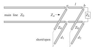
Fig. 13.10.1 Double stub tuner.
