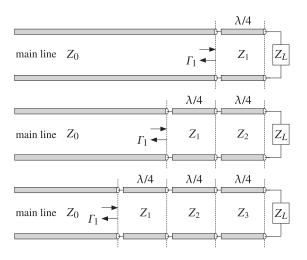
Fig. 13.3.1 One, two, and three-section quarter-wavelength transformers.
