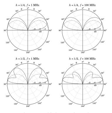
Fig. 22.3.5 Vertical dipole over imperfect ground
