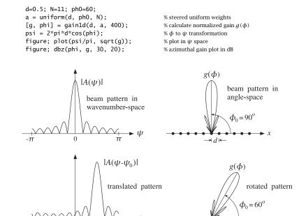
Fig. 22.9.1 Array steering or scanning by translation in wavenumber space.
