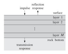
**Fig. 6.7.3** Seismic probing of earth's multilayer structure.
