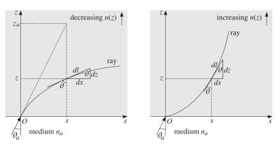
Fig. 7.15.1 Rays in an inhomogeneous medium.
