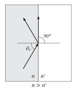
Fig. 7.5.1 Maximum angle of refraction and critical angle of incidence.
