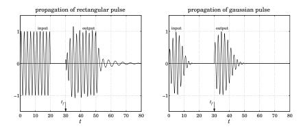
Fig. 3.4.3 Rectangular and gaussian pulse propagation.
