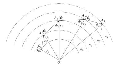
Fig. 7.15.6 Ray tracing in spherically stratified medium.
