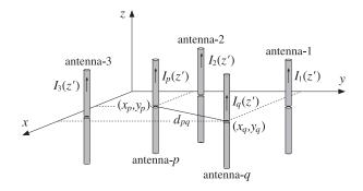
Fig. 25.5.1 Two-dimensional array of parallel dipoles.
