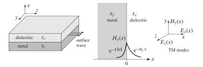
Fig. 10.2.1 Surface plasmon wave propagating along metal-dielectric interface.
