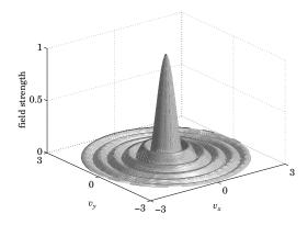
**Fig. 18.9.1** Radiation pattern of circular aperture ( $a = 3\lambda$ ).
