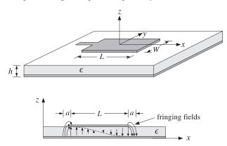
**Fig. 21.6.1** Microstrip antenna and *E*-field pattern in substrate.
