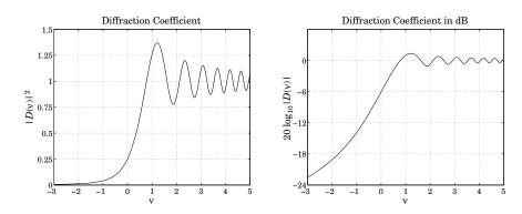
Fig. 18.14.2 Diffraction coefficient in absolute and dB units.
