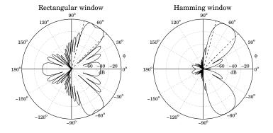
Fig. 23.5.1 Angular sector array design with Woodward-Lawson method.
