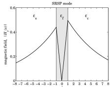
**Fig. 10.13.1** Magnetic field profiles, 2a = 20 nm film.
