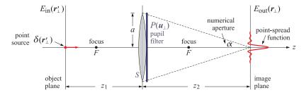
Fig. 20.7.1 Lens imaging system and its point-spread function.
