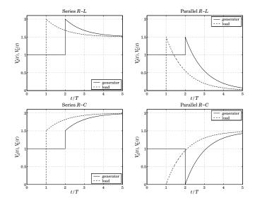
Fig. 11.15.4 Transient response of reactive terminations.
