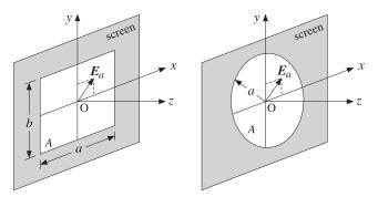
Fig. 18.7.1 Uniform rectangular and circular apertures.
