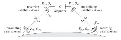
Fig. 16.10.1 Uplink and downlink in satellite communications.
