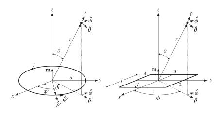
Fig. 17.8.1 Circular and square loop antennas.
