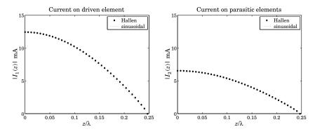
Fig. 25.7.1 Currents on driven and parasitic antennas.
