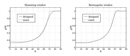
Fig. 23.5.2 Woodward-Lawson design of secant-squared array gain.
