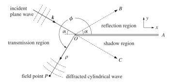
Fig. 18.15.2 Plane wave incident on conducting half-plane.
