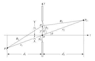
Fig. 18.13.2 Fresnel diffraction by rectangular aperture.
