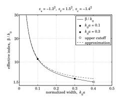
**Fig. 10.4.6** Effective index,  $\beta/k_0$ , versus normalized thickness,  $k_0a$ . Region 2.
