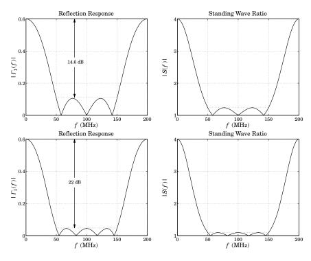
**Fig. 13.3.3** Three and four section transformers.
