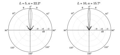
Fig. 17.7.6 Rhombic antenna gains in dB.
