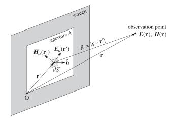
**Fig. 18.1.1** Radiated fields from an aperture.
