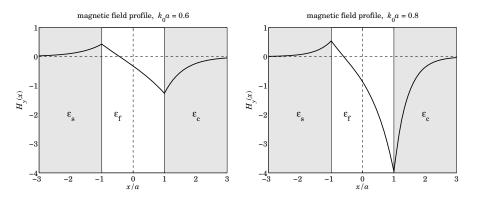
**Fig. 10.4.3** Magnetic field profiles,  $H_{\nu}(x)$  versus x for antisymmetric-like TM<sub>1</sub> mode.
