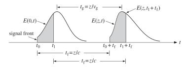
**Fig. 3.2.2** Shaded areas show causally related portions of input and propagated signals.
