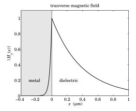
Fig. 10.2.2 Surface plasmon magnetic field profile.
