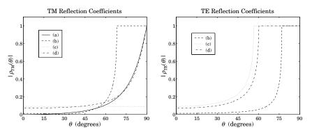
**Fig. 8.11.1** TM and TE birefringent Fresnel reflection coefficients versus incident angle.
