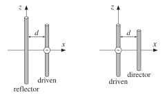
Fig. 25.6.2 The simplest Yagi-Uda arrays.
