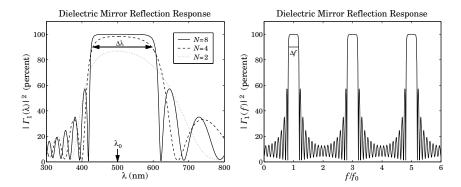
Fig. 6.3.2 Dielectric mirror with quarter-wavelength layers.
