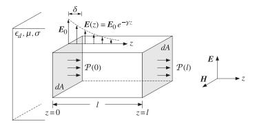
Fig. 2.6.1 Power flow in lossy dielectric.
