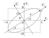
Fig. 2.5.2 General polarization ellipse.
