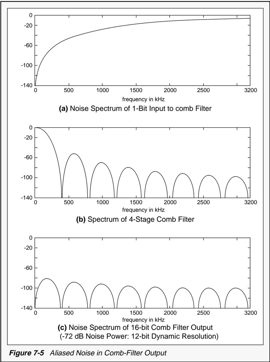
**Figure 7-5** Aliased Noise in Comb-Filter Output
