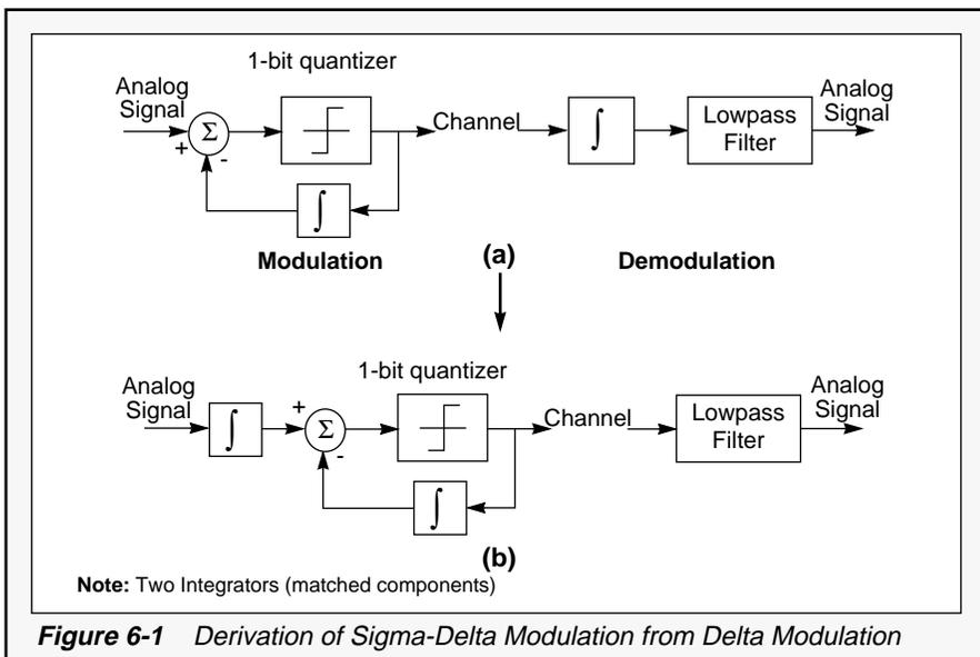
The arrangement shown in Figure 6-2 is called a *Sigma-Delta ( $\Sigma$ - $\Delta$ ) Modulator* [1]. This structure, besides being simpler, can be considered as being a “*smoothed version*” of a 1-bit delta modulator.
