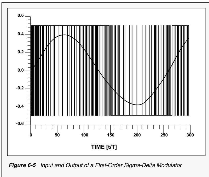
**Figure 6-5** *Input and Output of a First-Order Sigma-Delta Modulator*
