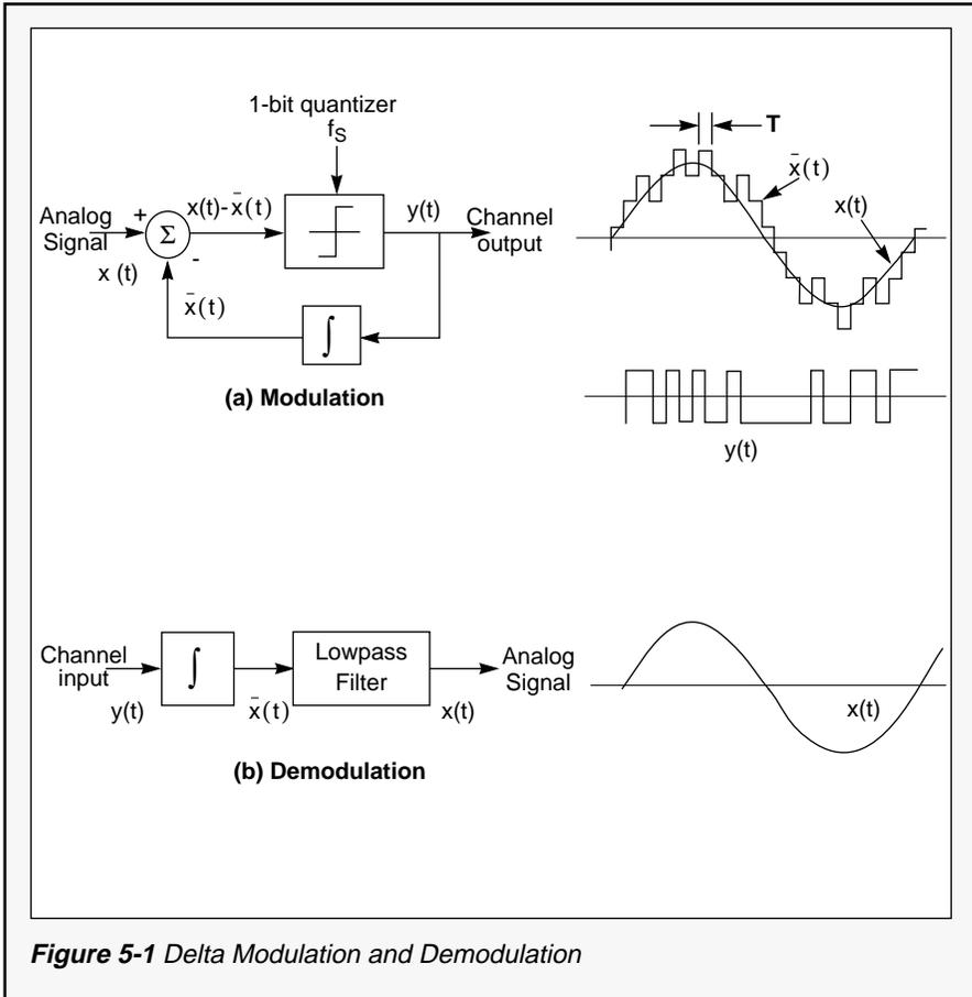
**Figure 5-1** Delta Modulation and Demodulation
