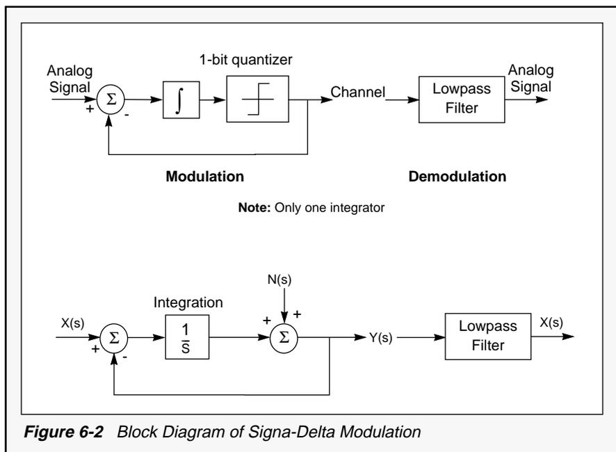
The name *Sigma-Delta* modulator comes from putting the integrator (sigma) in front of the delta modulator. Sometimes, the  $\Sigma$ - $\Delta$  modulator is referred to as an interpolative coder [14]. The quantization noise characteristic (noise performance) of such a coder is frequency dependent in contrast to delta modulation. As will be discussed further, this noise-shaping property is well suited to signal processing applications such as digital audio and communication. Like delta
