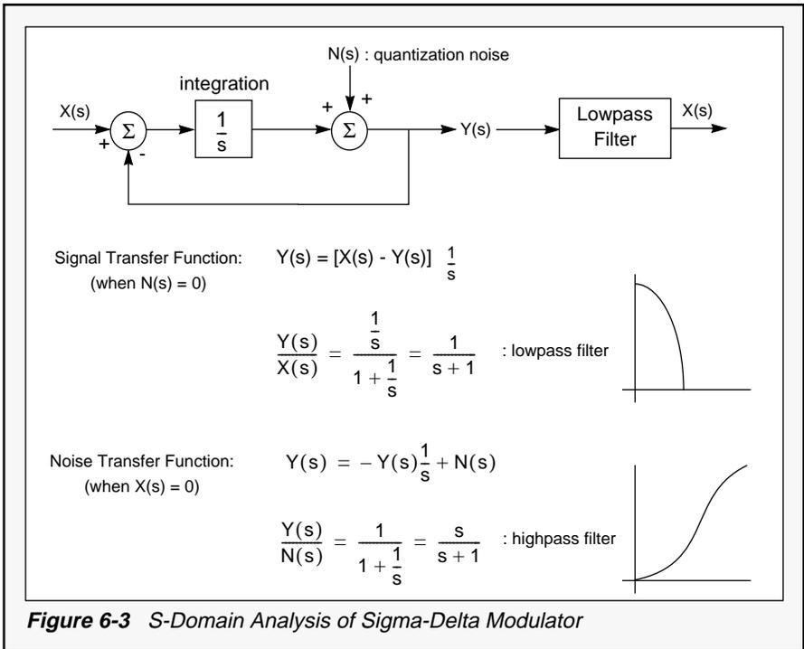
The noise-shaping principle is illustrated by a simplified "s-domain" model of a first-order  $\Sigma$ - $\Delta$  modulator shown in Figure 6-3. The summing node to the right of the integrator represents a comparator. It's here that sampling occurs and quantization noise is added into the model. The signal-to-noise (S/N)
