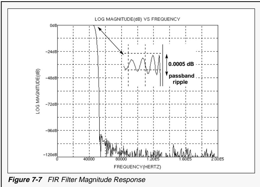
Although FIR filters take more time to perform the decimation filtering process than infinite impulse response (IIR) filters for the same passband and out-of-band frequency characteristics, FIR filters can be designed to have a linear-phase response which is required for high-end audio and instrumentation applications.
