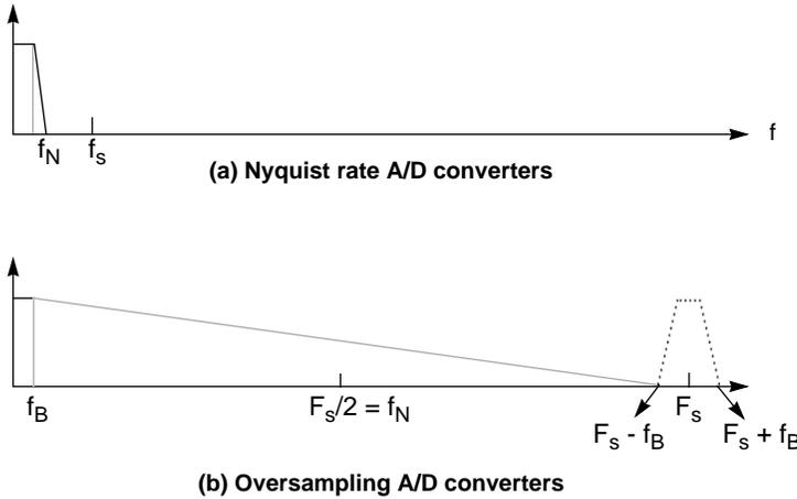
**Figure 4-3** Frequency Response of Analog Anti-Aliasing Filters
