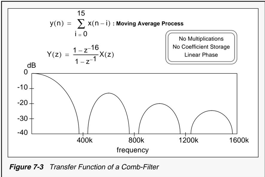
A single comb-filter stage usually does not have enough stop-band attenuation in the region of interest to prevent aliasing after decimation. However, cascaded comb-filters can be used to give enough stop-band attenuation. Figure 7-4 shows a structure of four cascaded comb filter sections and the resulting spectrum compared to lower order comb-filter stages. This realization needs eight registers for data and  $4(N+1)$  additions per input for computation.
