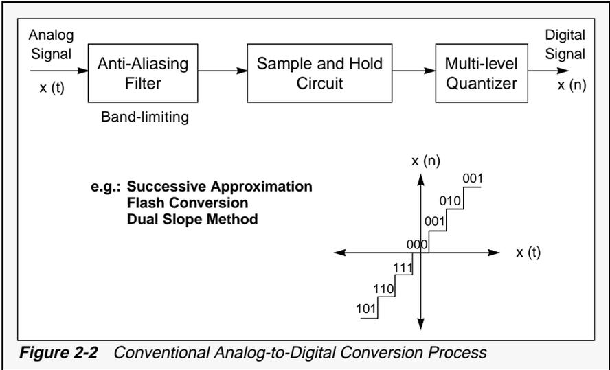
Figure 2-2 illustrates the conventional A/D conversion process that transforms an analog input signal  $x(t)$  into a sequence of digital codes  $x(n)$  at a sampling rate of  $f_s = 1/T$ , where  $T$  denotes the sampling interval. Since  $\delta(t - nT)$  in Eqn. 2-1 is a periodic function with period  $T$ , it can be represented by a Fourier series given by [5]:
