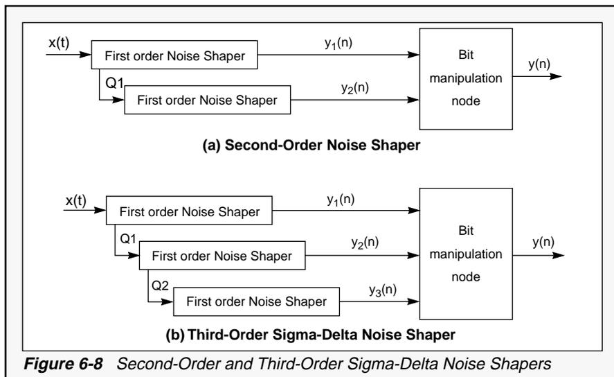
If the input signals to the second and third stage  $\Sigma$ - $\Delta$  loops are  $Q_1$  and  $Q_2$ , respectively, the quantization output for the second order  $\Sigma$ - $\Delta$  modulator is given by:
