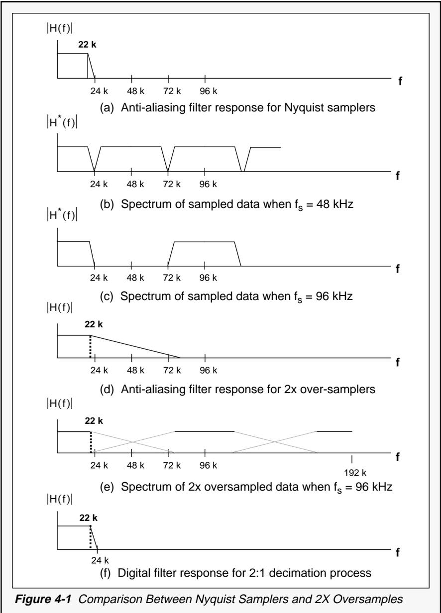
**Figure 4-1** Comparison Between Nyquist Samplers and 2X Oversamples
