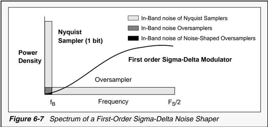
Figure 6-7 shows the spectrum of a first-order  $\Sigma\text{-}\Delta$  noise-shaper described in Figure 6-6. As shown in Figure 6-7, the baseband (up to  $f_B$ ) noise of the  $\Sigma\text{-}\Delta$  converters appears to be much smaller than Nyquist samplers or delta modulators. However, for the first order modulator discussed, the baseband noise can not reach below the -96 dB signal-to-noise ratio needed for 16-bit A/D converters.
