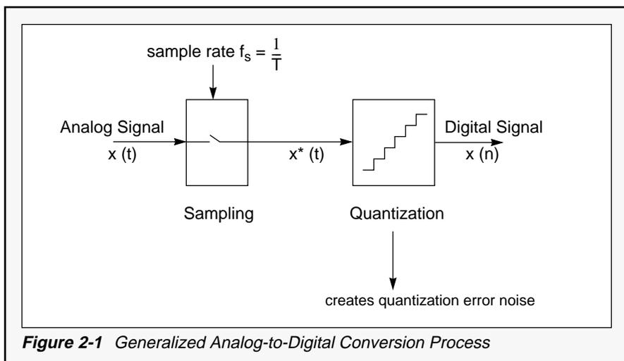
**Figure 2-1** Generalized Analog-to-Digital Conversion Process
