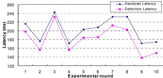
Fig. 8. Detection and Handover latency of SFB-MIP, FA-HA latency=400ms, with MIH support. (Notice the scale difference of the vertical axis compared with Fig.7)
