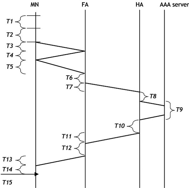
Fig. 2. Timing diagram for handover using Mobile IP
