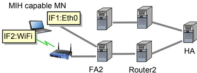
Fig. 3. MN with 2 interfaces connecting to a single FA
