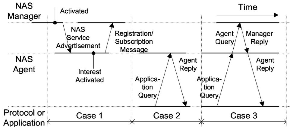
Figure 3. Communications between NAS components.
