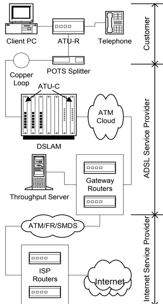
Figure 1: ADSL deployment architecture
