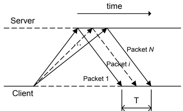
Figure 3: Upstream scheme of bandwidth measurement
