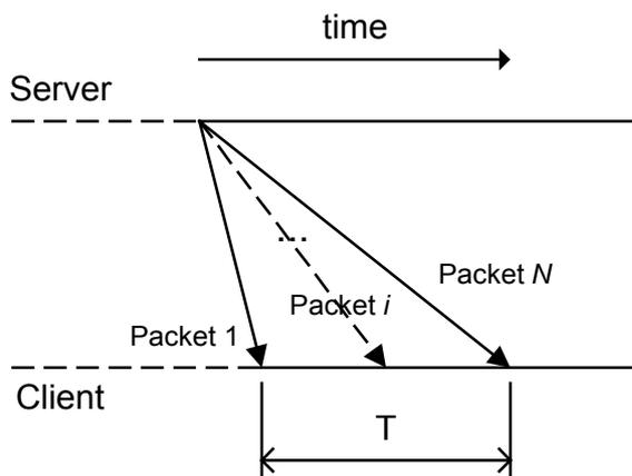
**Figure 4:** Downstream scheme of bandwidth measurement
