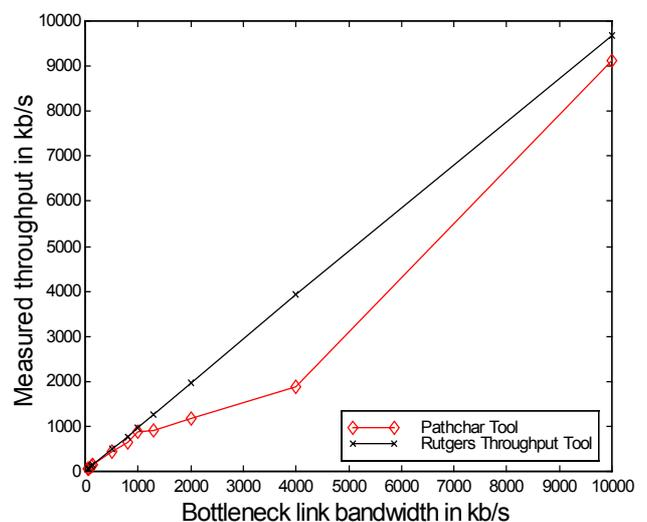
Figure 6: Comparison of tools for bandwidth measurement
