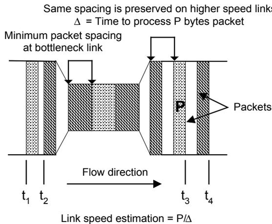
Figure 2: Packet-pair technique for bandwidth measurement
