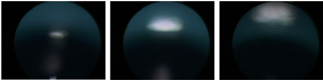
Figure 8: Illumination addressing. The illumination aperture is moved so that the incident ray changes from the top center of the mirror (left image) toward the bottom center of the mirror (right image). Notice the specularity moves in the opposite direction as one would expect from the mirror geometry.
