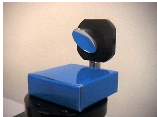
Figure 5: Off-axis concave parabolic mirror used in prototype with a sample (glossy blue cardboard) at focus.
