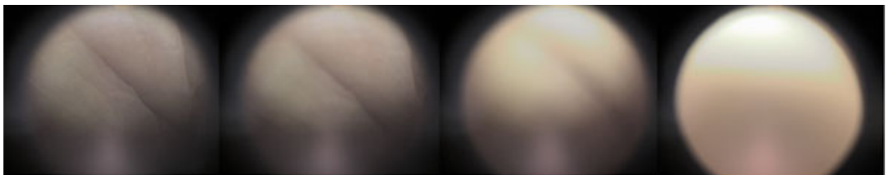
Figure 10: Images from camera as mirror focuses on skin surface. When the focal point is above the surface, surrounding texture is discernible. The images from left to right depict the camera view as the focal point approaches the surface. These views can be used to navigate the mirror focus to the desired surface point.
