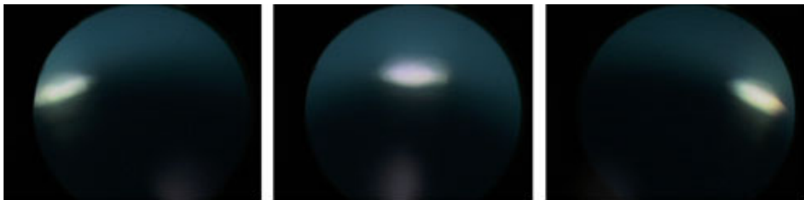
Figure 9: Illumination addressing. The illumination aperture is moved so that the incident ray changes from the right side of the mirror (left image) to left side (right image). Notice the specularity moves in the opposite direction.
