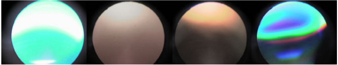
Figure 7: Images of the aggregate BRDF obtained for four samples. From left to right the samples are (1) glossy blue cardboard, (2) skin surface of the author's hand, (3) diffuse brick, (4) the surface of a CD (compact disk).
