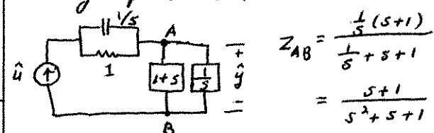
$$\begin{aligned} Z_{AB} &= \frac{\frac{1}{s+1}}{\frac{1}{s+1} + \frac{1}{s+1}} \\ &= \frac{s+1}{s^2 + s + 1} \end{aligned}$$
