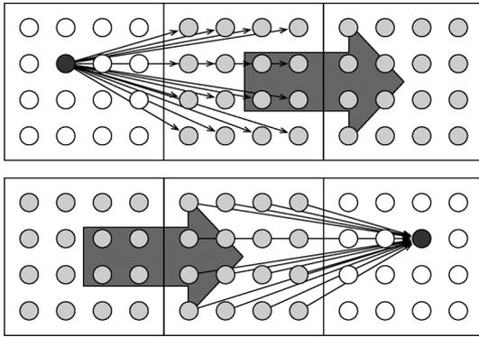
Fig. 2. Routing flow in the local mobility model. As illustrated on top, for node  $i$  to send to node  $j$ , it evenly divides the flow and sends it to all node in the adjacent square in the L-shaped path. Each node in the adjacent square routes that flow uniformly to every node in the next square in the path. At the end of the route, as illustrated on the bottom, the nodes in the square adjacent to the destination  $j$  transmit their received flows directly to  $j$ .
