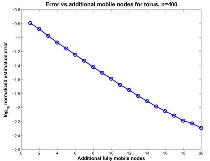
Fig. 7. Adding a few mobile nodes to a static grid can exponentially decrease the estimation error for a fixed number of iterations (20 000).
