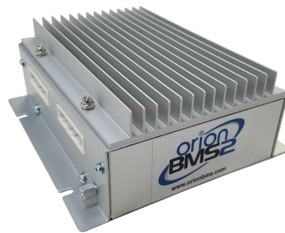
Figure 1 → The Orion BMS, the system currently in use for the RFR racecar.
