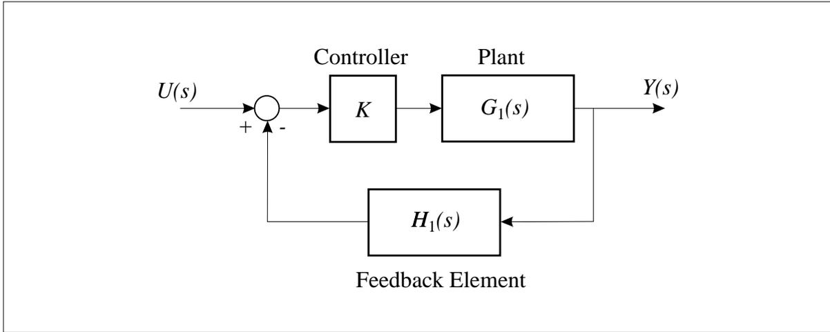
Figure 7.2: Feedback control system with a static controller in the direct path
