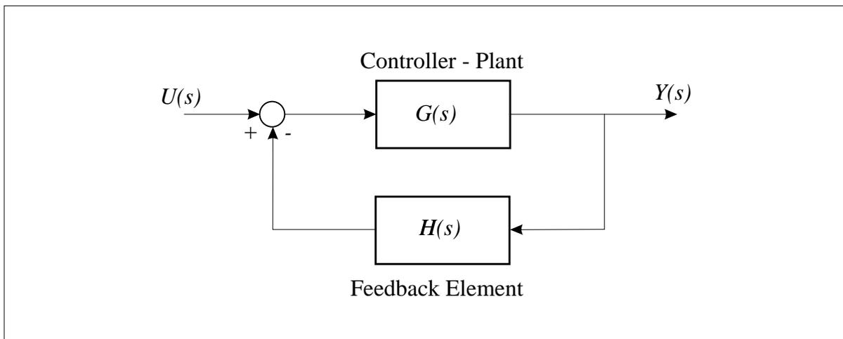
Figure 7.1: Block diagram of a feedback control system
